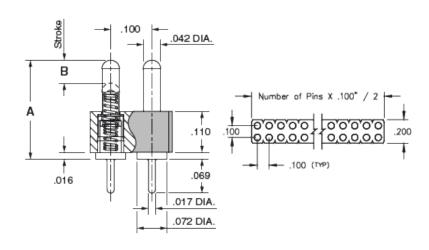
**Description:** Interconnect SLC Header Spring-Loaded Header Vertical Mount Through-Hole
