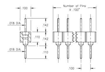
**Description:** Interconnect Header Solder Tail Pin Header .018" (0,46mm) Pin Head Single Row Through Hole Plating Code: 10 Shell Plating: 10 µ" Gold over 100 µ" Nickel
