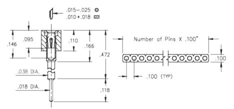
**Description:** Interconnect Socket Elevated Strip Socket Accepts .015" - .025" (0,38 - 0,635 mm) dia leads Single Row Through Hole Plating Code:
