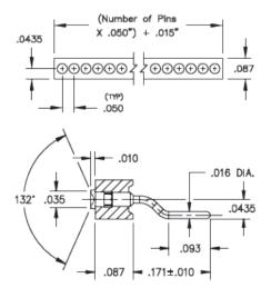
Description: Interconnect Target Connector Spring-Loaded Header Horizontal Mount Target with **Concave Face** Single Row Through Hole Plating Code: 10 Shell Plating:
