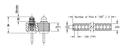
**Description:** Interconnect SLC Header Spring-Loaded Header Vertical Mount Through-Hole Double Row Through Hole Plating Code: 22 Shell Plating: 20µ" Gold over 100µ" Nickel Inner Spring Plating: 10µ" Gold
