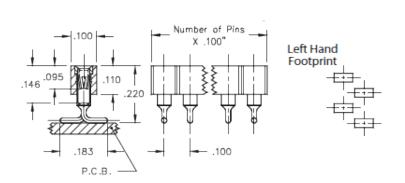
Interconnect Socket Surface Mount Socket Accepts .015"- .025" (0,38 - 0,635 mm) dia leads Single Row Surface Mount Plating Code: 93 Shell Plating: 200 μ" Tin/Lead(93/7) over 100 μ" Nickel Inner Contact Plating:
