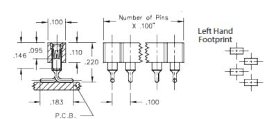
**Description:** Interconnect Socket Surface Mount Socket Accepts .015" - .025" (0,38 - 0,635 mm) dia leads Single Row Surface Mount
