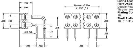
**Description:** Interconnect Target Connector Spring-Loaded Header Right Angle Mount Target Double Row Through Hole Plating Code: Shell Plating: 10  $\mu$ " Gold over 100  $\mu$ " Nickel
