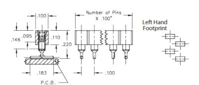
**Description:** Interconnect Socket Surface Mount Socket Accepts .015" - .025" (0,38 - 0,635 mm) dia leads Single Row Surface Mount **Plating Code:**
