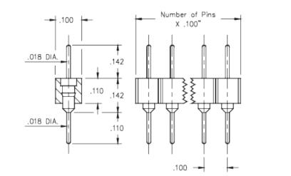
**Description:** Interconnect Header Solder Tail Pin Header .018" (0,46mm) Pin Head Single Row Through Hole Plating Code: 90 Shell Plating: 200 μ" Tin/Lead(93/7) over 100 μ" Nickel
