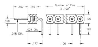
**Description:** Interconnect Header Right Angle Pin Header .018" (0,46mm) Pin Head Single Row Through Hole Plating Code: 10 Shell Plating: 10 µ" Gold over 100 µ" Nickel
