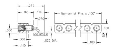
**Description:** Interconnect Socket Horizontal Mount Socket Accepts .025" - .037" (0,635 - 0,94 mm)dia leads Single Row Surface Mount **Plating Code: Shell Plating:** 200 μ" Tin (matte finish) over 100 μ" Nickel Inner Contact Plating:
