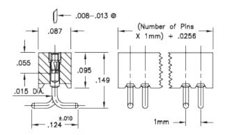
Interconnect Socket Surface Mount Socket Accepts .008" - .013" (0,203 - 0,33 mm) dia leads Single Row Surface Mount **Plating Code:** Shell Plating: 10 μ" Gold over 100 μ" Nickel Inner Contact Plating: 30 μ" Gold over 50 μ" Nickel
