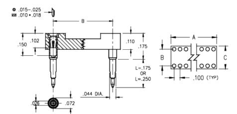
**Description:** DIP Dual In Line Socket Solderless Press-Fit Standard Tail Open Frame Through Hole Plating Code: Shell Plating: 10 μ" Gold over 100 μ" Nickel Inner Contact Plating:
