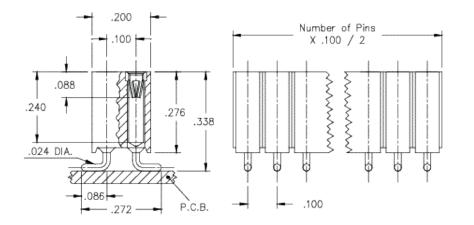
**Description:** Interconnect Socket Surface Mount Socket Accepts .025" - .037" (0,635 - 0,94 mm)dia leads Double Row Surface Mount **Plating Code:** 43
