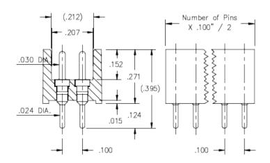
**Description:** Interconnect Header Shrouded Pin Header .030" (0,76mm) Pin Head Double Row Through Hole Plating Code: 10
