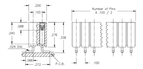
**Description:** Interconnect Socket Surface Mount Socket Accepts .025" - .037" (0,635 - 0,94 mm)dia leads Double Row Surface Mount **Plating Code: Shell Plating:**
