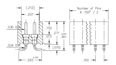
**Description:** Interconnect Header Shrouded Pin Header .030" (0,76mm) Pin Head Double Row Through Hole **Plating Code:** 10 **Shell Plating:** 10 µ" Gold over 100 µ" Nickel
