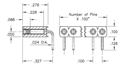
Interconnect Socket Right Angle Socket Accepts .025"- .037" (0,635 - 0,94 mm)dia leads Single Row Through Hole Plating Code: 43 Shell Plating: 200 µ" Tin (matte finish) over 100 µ" Nickel Inner Contact Plating: 30 µ" Gold over 50 µ" Nickel
