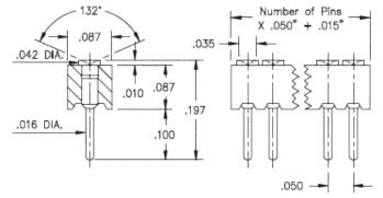
Description: Interconnect Target Connector Spring-Loaded Header Vertical Mount Through Hole Target with Concave Face Single Row Through Hole Plating Code: 10 Shell Plating:
