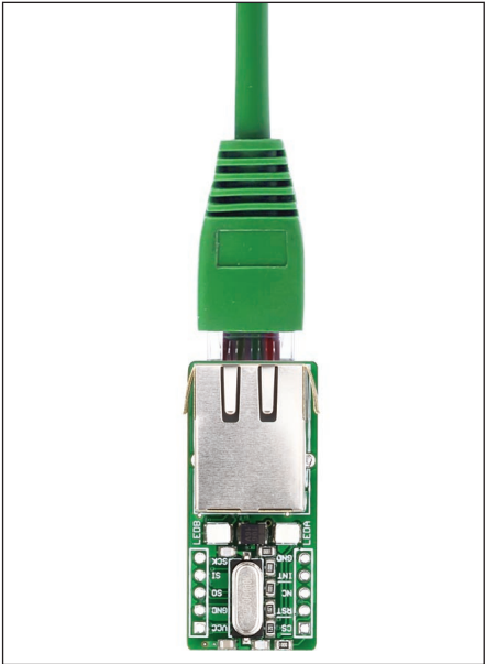
Figure 3: mikroETH connected to a ethernet cable
