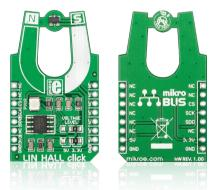
LIN HALL click<sup>™</sup> is a simple solution for adding a linear Hall sensor to your design. It carries an MLX90242 linear Hall sensor IC (with built-in active error correction circuitry) and an MCP3201 12-bit ADC. LIN HALL click™ communicates with the target board through the **mikroBUS**<sup>™</sup> SPI lines (CS, SCK, MISO). The board is designed to use either a 3.3V or 5V power supply.
