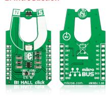
BI HALL click<sup>™</sup> is a simple solution for adding a bipolar Hall switch to your design. It carries the Melexis US2882 bipolar Hall-effect switch and a 74LVC1T45 single bit, dual supply transceiver. BI HALL click<sup>™</sup> communicates with the target board through the mikroBUS<sup>™</sup> INT line. The board is designed to use either a 3.3V or 5V power supply (which also defines the logic level of the output signal).
