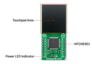
On the front side of the Touchpad 3 Click, there is a clearly defined field that represents a touchpad area. This area is a matrix of conductive electrodes on the PCB, electrically isolated from each other, arranged as rows and columns of X and Y. An electrode consists of multiple diamond-shaped elements, each connected to the next with a conductive neck.
