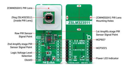
Combined with the ZSLM323511, the PIR 2 Click also integrates the ZCWM05GIV1 PIR lens, made from high-density polyethylene. This lens ensures maximum IR transmissivity with welldefined beam patterns. It clips directly into the Click board over the ZSLM323511 sensor, simplifying mechanical design.
