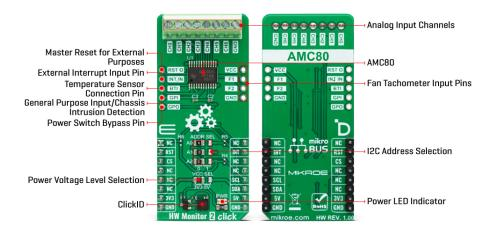
This Click board™ communicates with MCU using the standard I2C 2-Wire interface to read data and configure settings with a maximum frequency of 400kHz. The AMC80 includes an analog filter on the I2C lines that improves noise immunity and supports the timeout reset function on SDA and SCL pins, preventing I2C bus lockup. Also, the AMC80 allows choosing the least significant bits (LSB) of its I2C slave address using the SMD jumpers labeled ADDR SEL.
