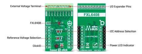
Expand 16 Click uses a standard 2-wire I2C interface to communicate with the host MCU, supporting clock frequency up to 400kHz. The I2C address can be selected over the ADDR SEL jumper. The FXL6408 has three reset options: power-on reset, over the software, and the RST pin by writing the logic LOW. When the event occurs, the I/O expander will assert the host MCU over the interrupt INT pin.
