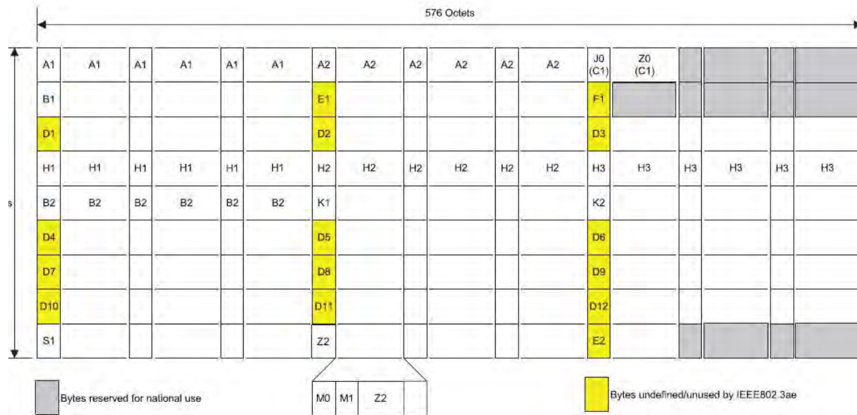
Figure 14 • STS-192c/STM-64 Section and Line Overhead Structure
