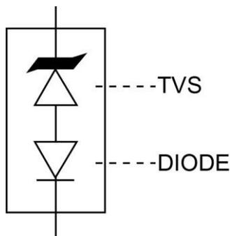
**Figure 6-2.** Optional Unidirectional Configuration (TVS and Separate Rectifier Diode in Parallel)
