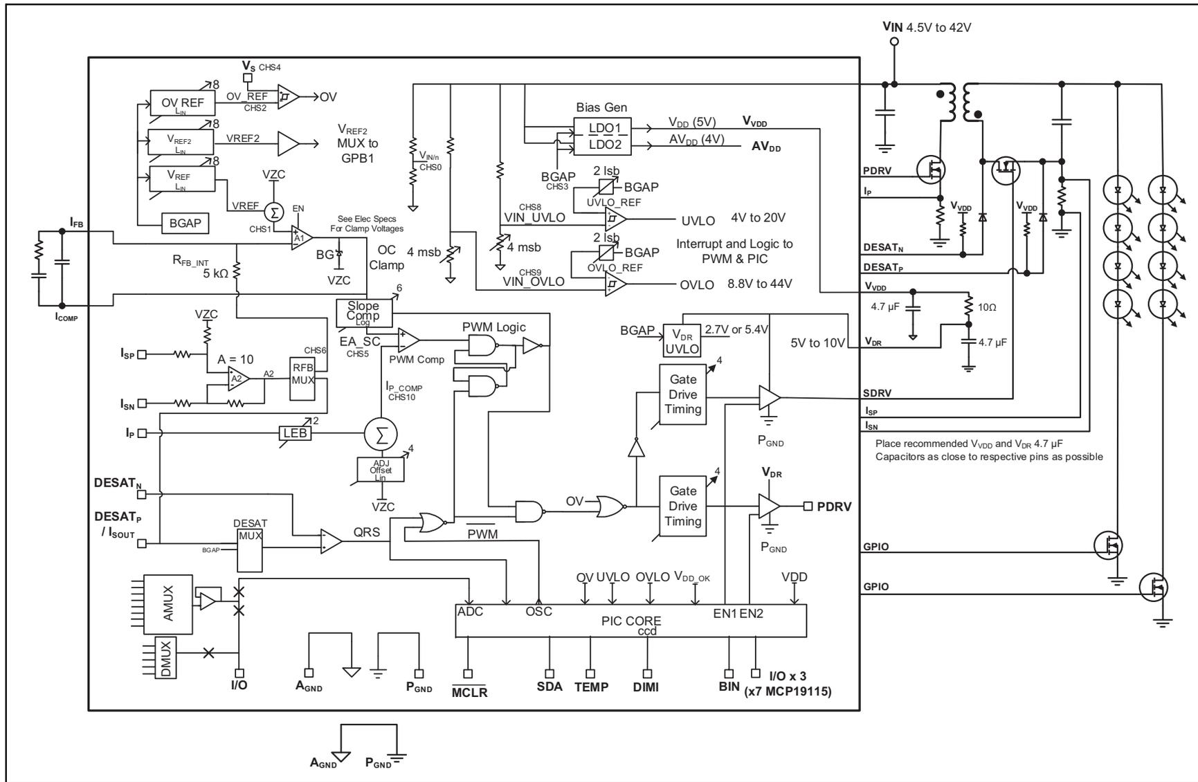
Place recommended V<sub>VDD</sub> and V<sub>DR</sub> 4.7 μF Capacitors as close to respective pins as possible
