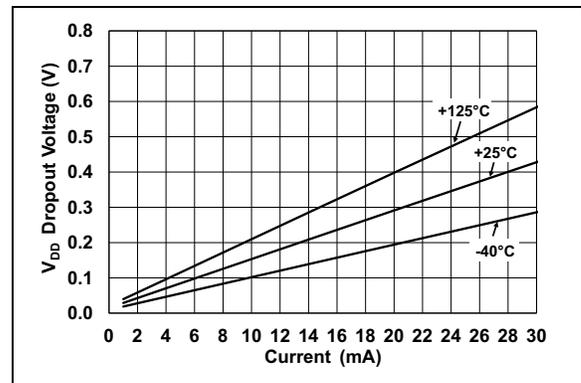
**FIGURE 7-5:**  $V_{DD}$  Dropout Voltage vs. Output Current (mA).
