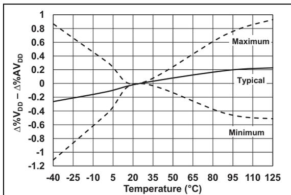
**FIGURE 7-15:**  $V_{DD}$  vs.  $AV_{DD}$  Temperature Drift Tracking.
