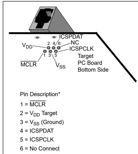
Another connector often found in use with the PICKit™ programmers is a standard 6-pin header with 0.1 inch spacing. Refer to [Figure 30-2](#).
