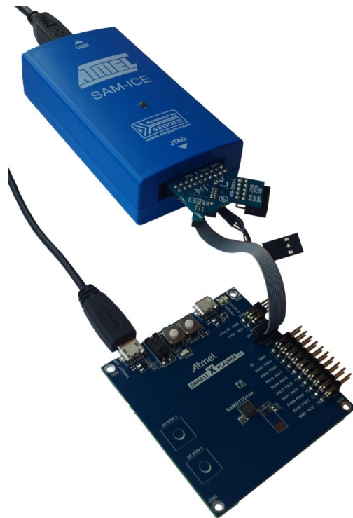
Figure 5-7. SAM-ICE using an Atmel-ICE Adapter
