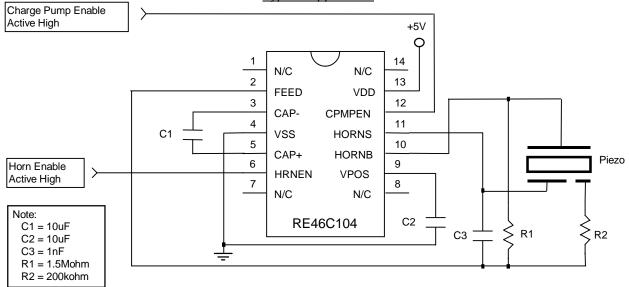
**Piezoelectric Horn Driver and Voltage Converter** Product Specification
