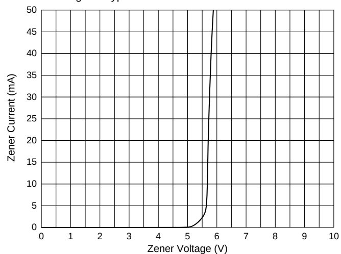
Fig. 5 - Typical Zener Breakdown Characteristics
