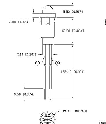
PANEL HOLE: Ø0.250" PANEL THICKNESS: 0.030" MIN.
