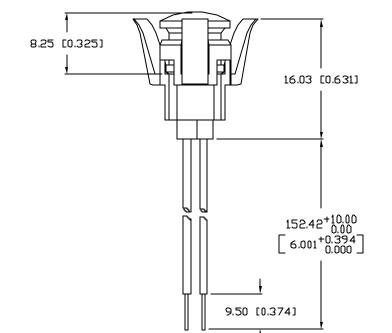
PANEL HOLE SIZE: 7.93 [0.312] TO 8.05 [0.317]. PANEL THICKNESS: 0.51 [0.020 TO 2.03 [0.080].
