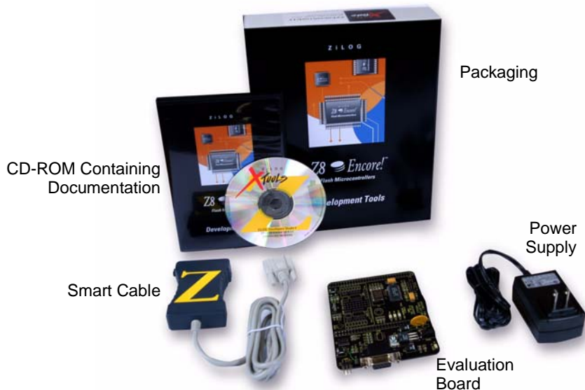
Figure 1. Z8 Encore! XP ® MCU Development Kit Contents
