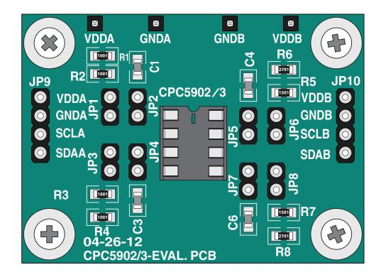
The CPC5902G/5903G Evaluation Board can be used to isolate an I<sup>2</sup>C bus, and to evaluate the performance obtainable when communicating between the user's I<sup>2</sup>C devices. The 8-pin DIP socket can be populated with either a CPC5902G (for both SCL and SDA bidirectional) or with a CPC5903G (for SDA bidirectional, SCL sideA to sideB only).
