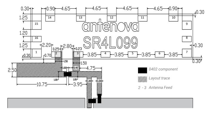
1 • 7 • 9 • 15 copper pads: 1.5 × 2.0 (mm) Others copper pads: 1.0 × 2.0 (mm)
