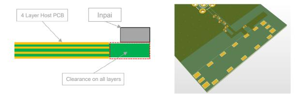
The Inpai antenna is placed on the left-hand corner of the host PCB following the drawing showing the exact placement of the antenna. It is important to not have any tracks or ground plane on both sides of the antenna, the antenna performance will be diminished if there are any tracks inside the clearance area (apart from the tracks shown in the drawing).
