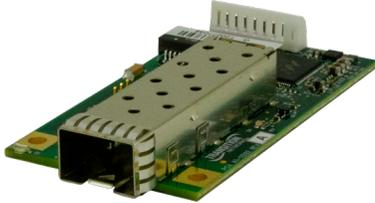
The AP-GET-SFP-01 is a 10/100/1000 Ethernet media converter that provides cost effective, entry-level media conversion between 10/100/1000Base-T ports and 100/1000Base-X fiber ports. Designed as an embedded solution that can be mounted internally in Tempest rated computer and networking equipment such as VoIP Phones, Workstations, Thin Clients, Printers, Monitors and similar devices. Government agencies like Intelligence, Defense, and Foreign Affairs generally
