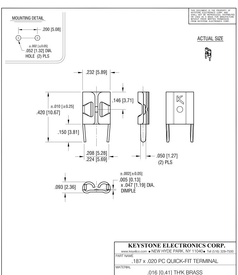
DRN BY DATE FINISH 4.15.09 В TIN NICKEL PLATE 9.18.20 CHANGE AS PER ECN 20-082 APP'D SCALE RH 4X Α 11.25.19 CHANGE AS PER ECN 19-090 TOLERANCES INCH [MM] CODE DWG NO.  $\pm .005 [\pm 0.13]$ DECIMAL 3578 C ANGULAR ± 1° DATE **DESCRIPTION** REV. UNLESS OTHERWISE SPECIFIED
