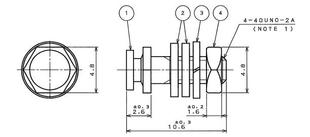
NOTE 1.THESE PARTS OF NO.2~NO.4 WERE ASSEMBLED TO BE ATTACHED.
