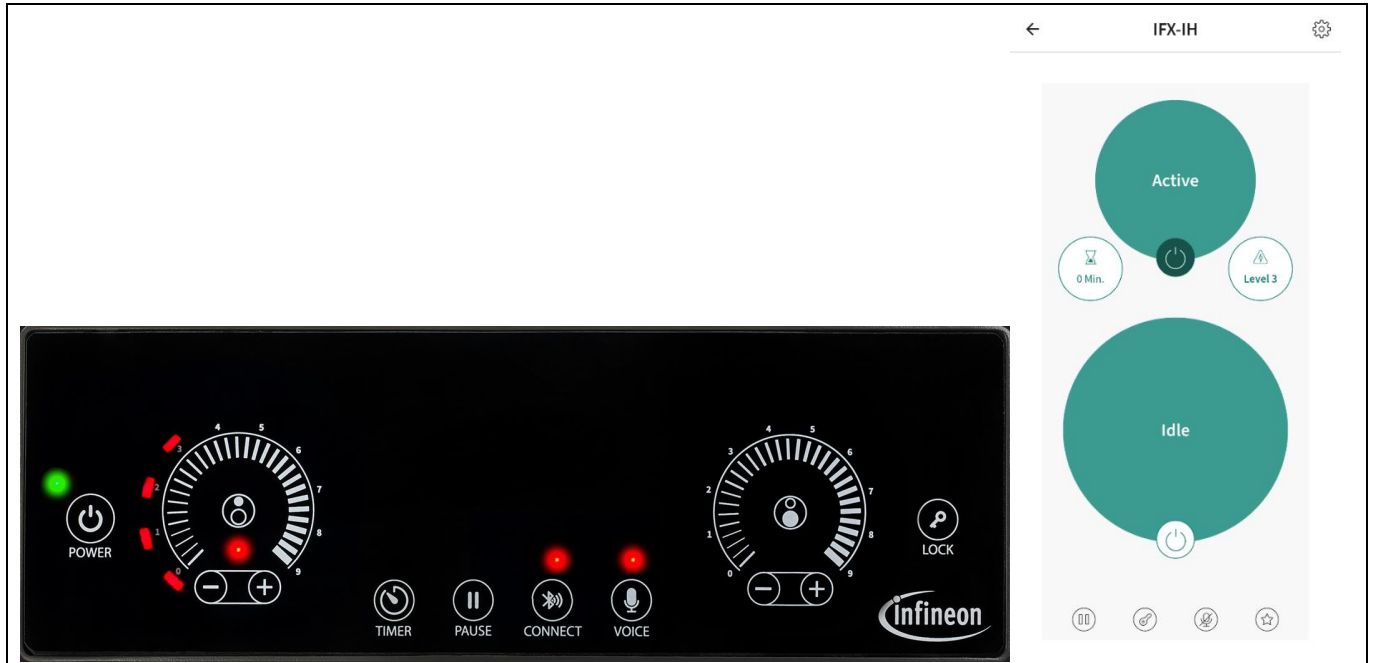
Figure 12 Small hob power level set to power level 3.
