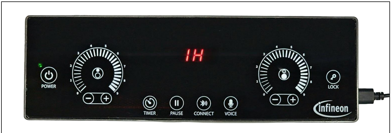
Figure 117 HMI & System Control Board in independent mode
