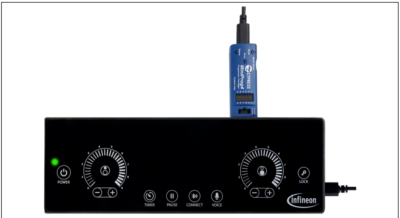
Figure 23 HMI & System Control Board debug interfaces - MiniProg4 and USB (power & debug console)
