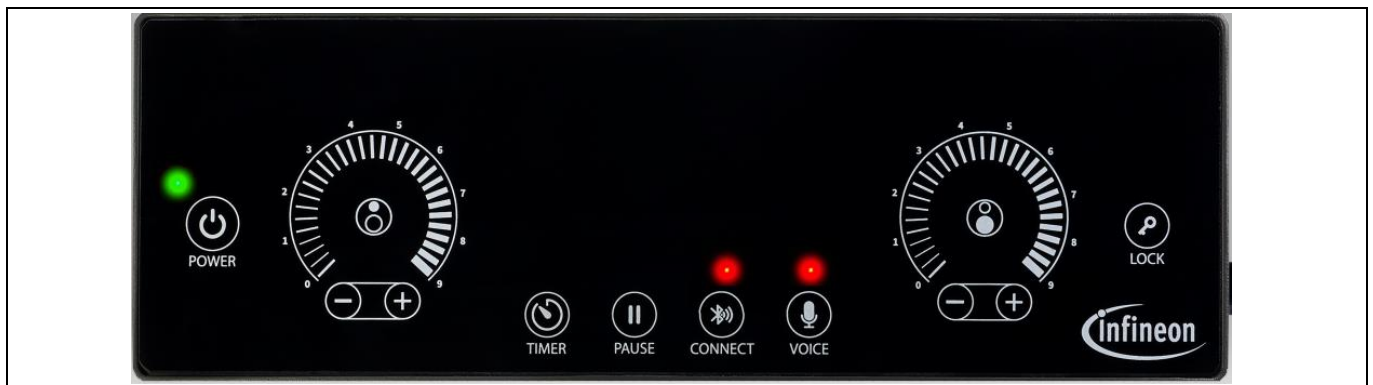
Figure 8 Smart induction cooktop in idle state with voice and connectivity enabled
