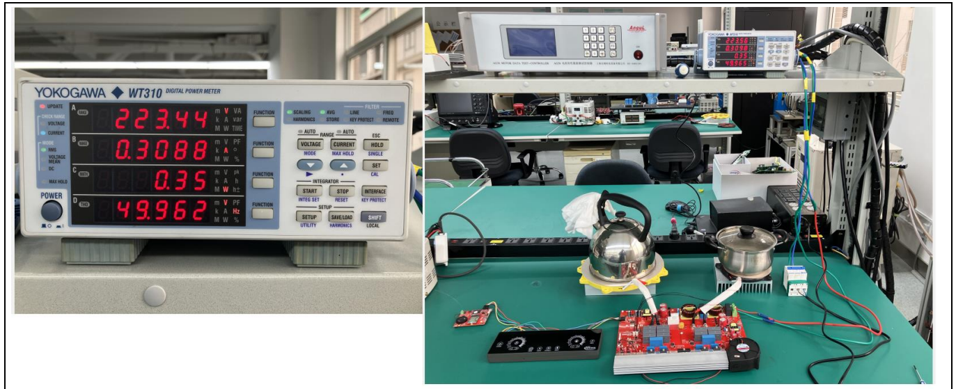
Figure 94 Standby power consumption of Smart Induction Cooktop Reference Design
