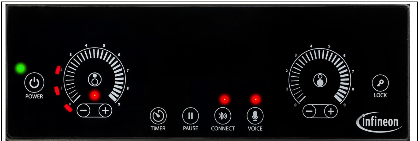
Figure 14 Small hob power level set to power level 2
