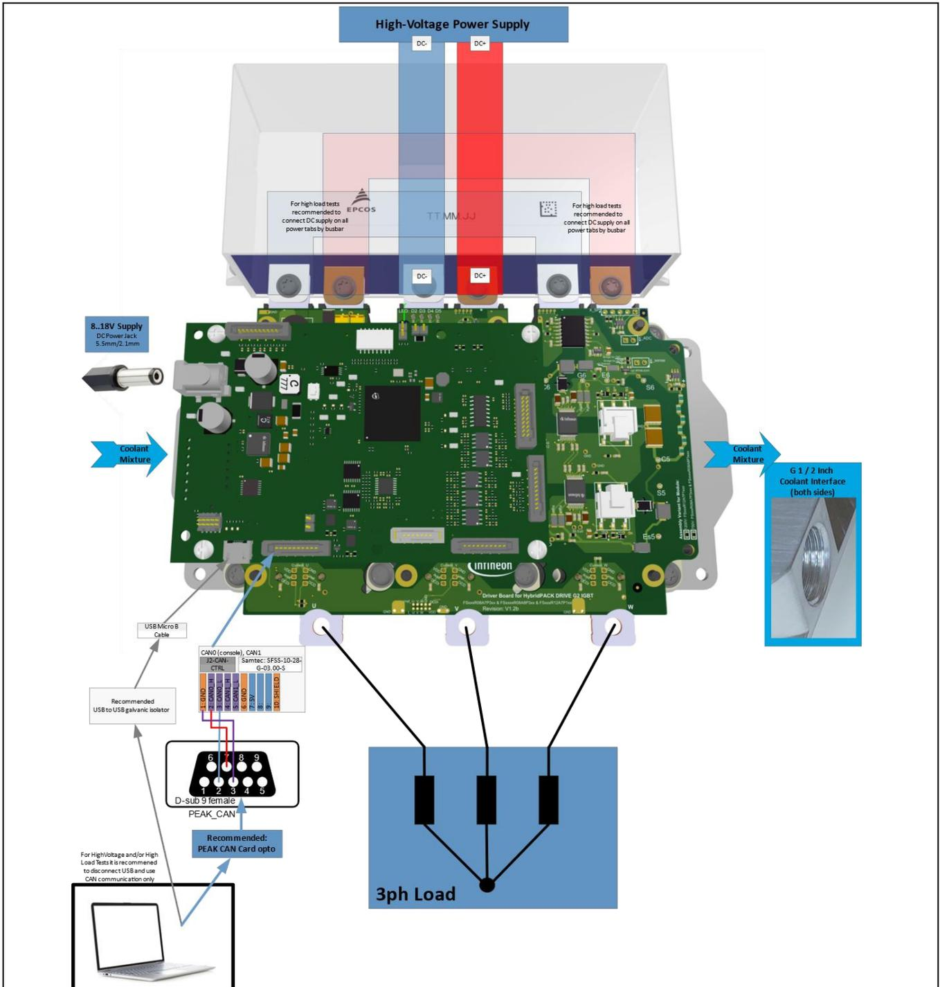
Figure 7 Typical setup for Inverter Load Tests.
