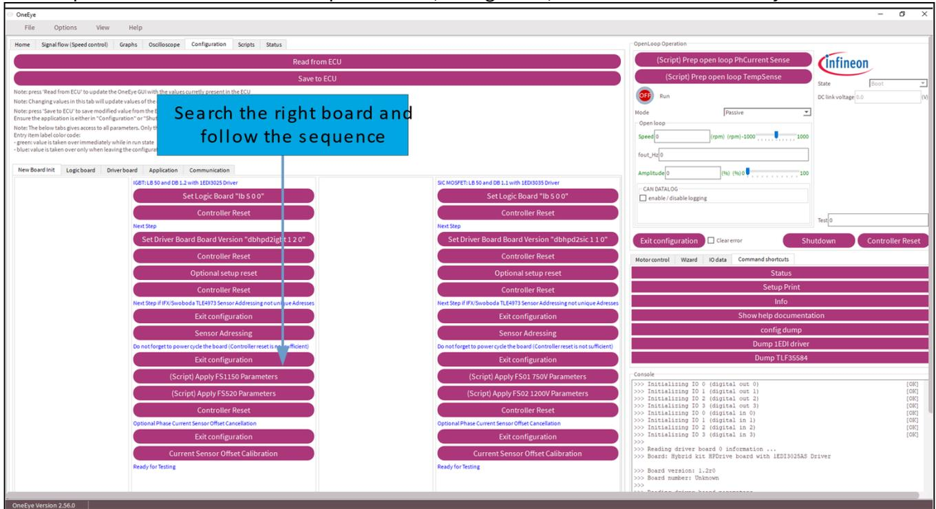
Figure 15 OneEye GUI for New Board Init sequence.
