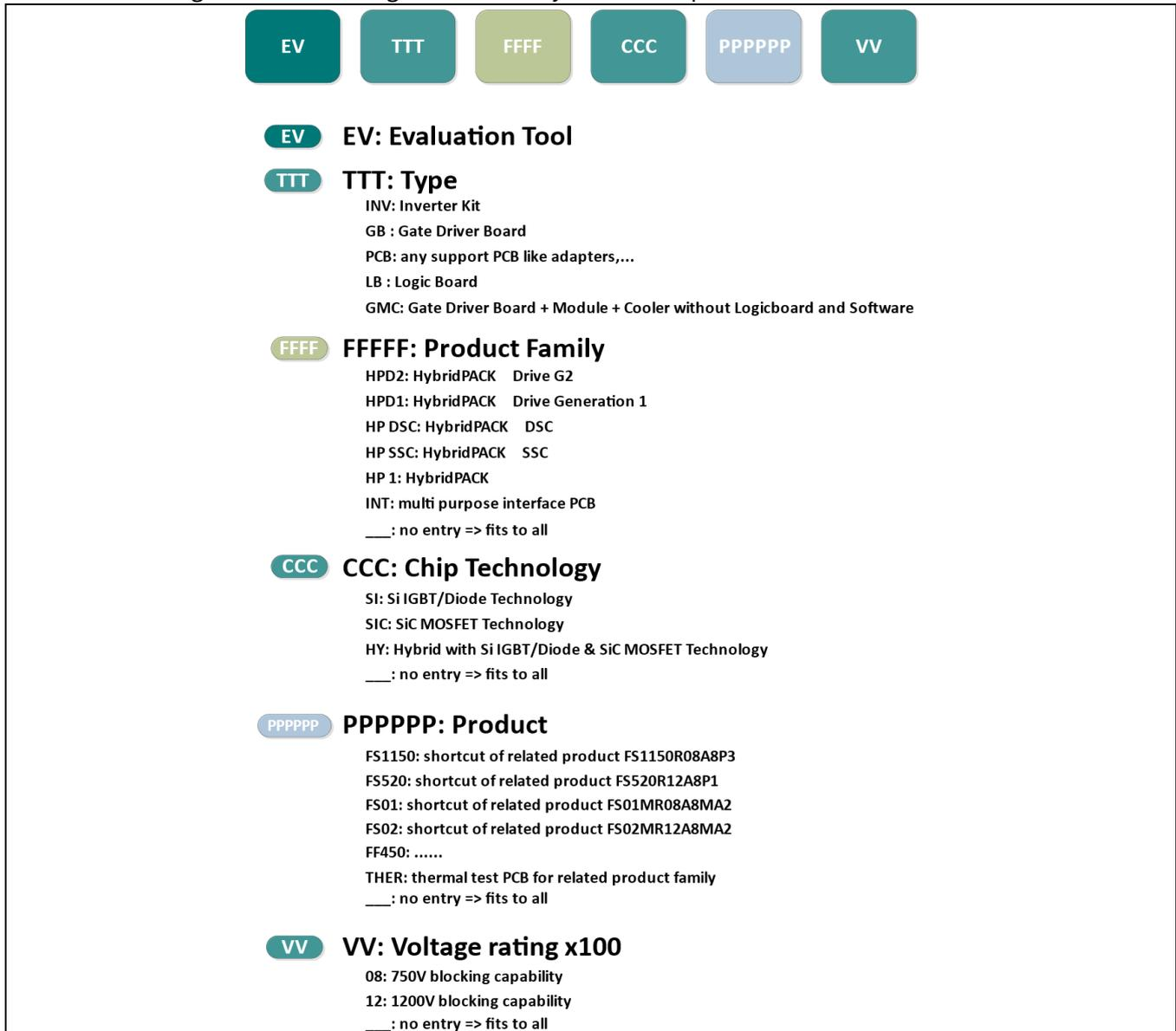
Figure 3 Type designation tree for the HybridPACK™ power module evaluation tools.
