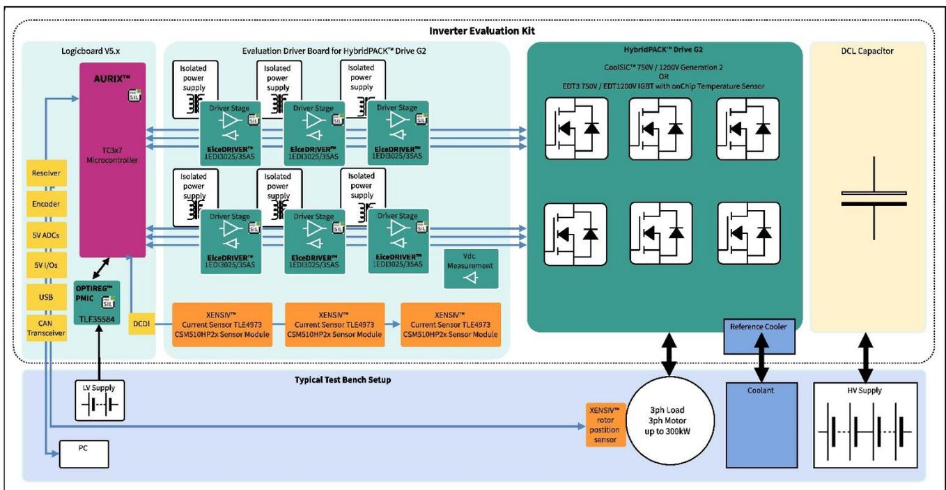
**Figure 1 Block Diagram of the Inverter Evaluation Kits for HybridPACK™ Drive G2 power modules**
