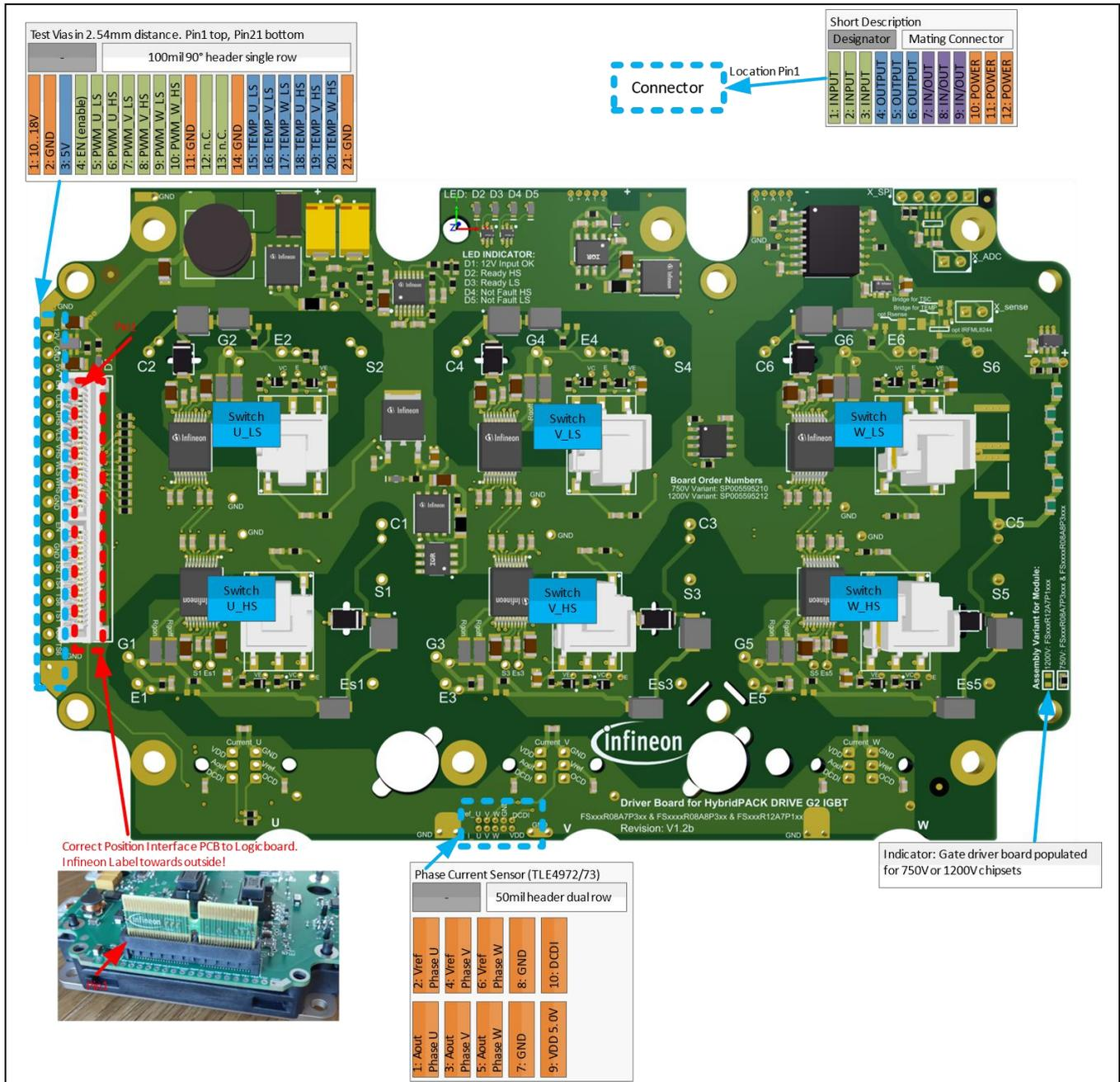
Figure 5 Connectors of Gate Driver Boards (IGBT Versions).
