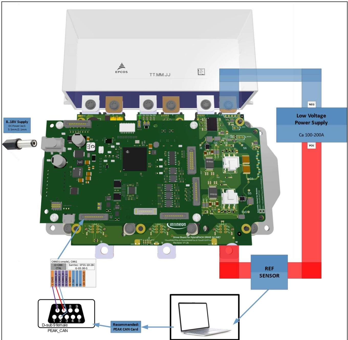
Figure 12 Setup for Gain Parameter Calibration of the Current Sensors (shown only example for phase W).
