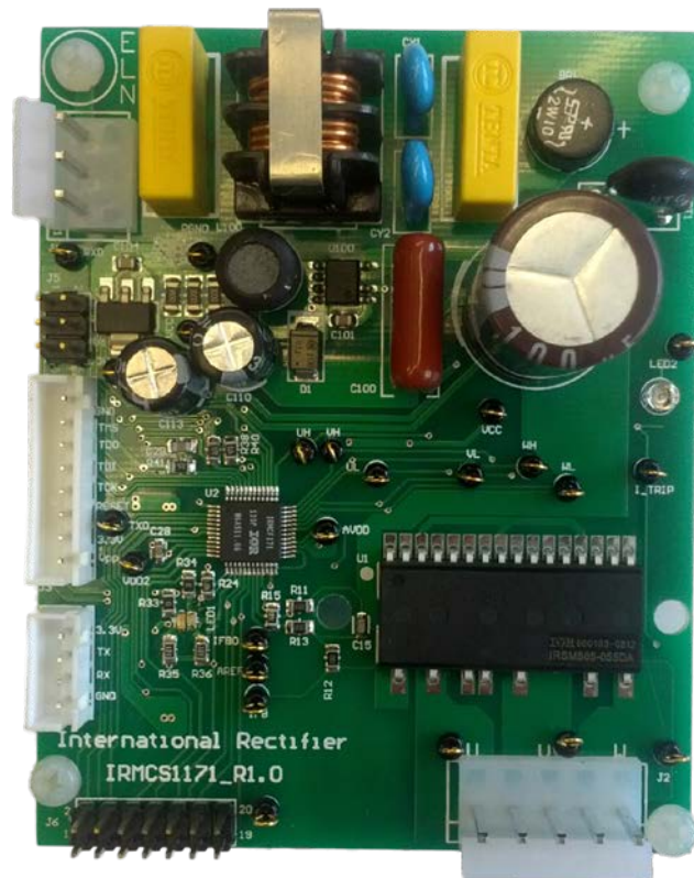
Figure 4: Reference design board featuring the μIPM™-DIP module and the iMotion™ IRMCF171 digital control IC
