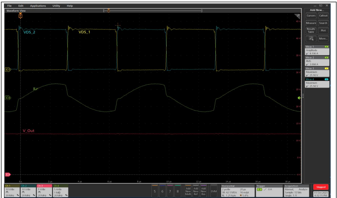
Figure 29 LLC in steady-state condition when running at 50 percent load
