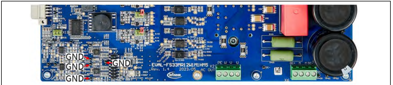
Figure 4 Relevant parts for offset adjustments
