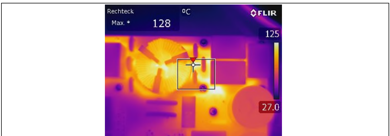
Figure 26 Thermal image of input area
