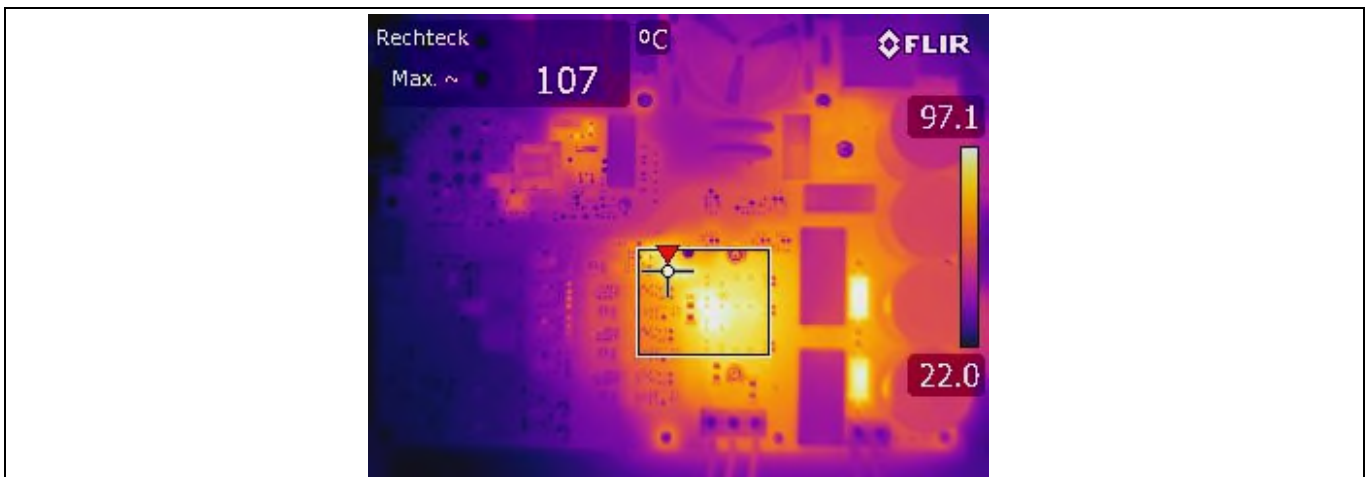
Figure 29 Thermal image of evaluation board at 100 kHz switching frequency
