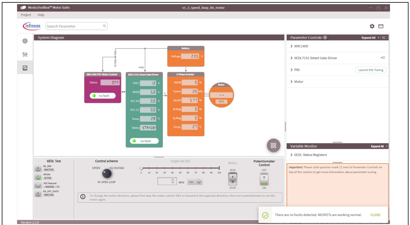
Figure 44 GUI: Off-state diagnostics without fault
