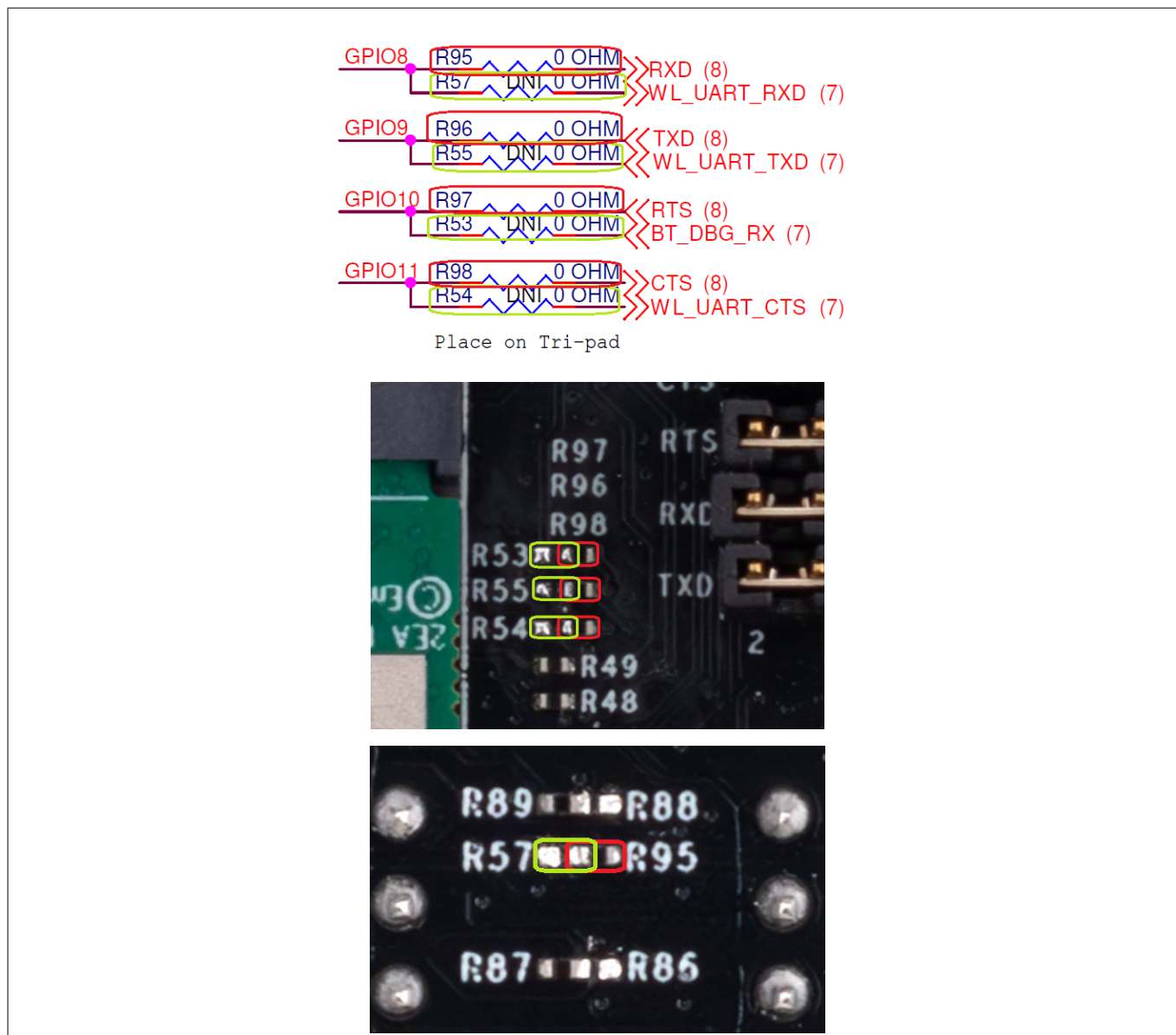
Figure 24 WL UART interface rework
