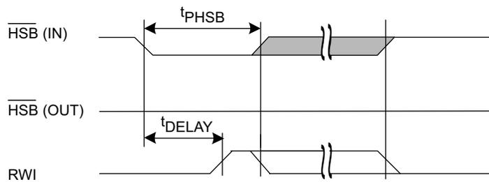
$\overline{\text{HSB}}$  pin is driven HIGH to  $V_{CC}$  only by Internal 100 K $\Omega$  resistor,  $\overline{\text{HSB}}$  driver is disabled
