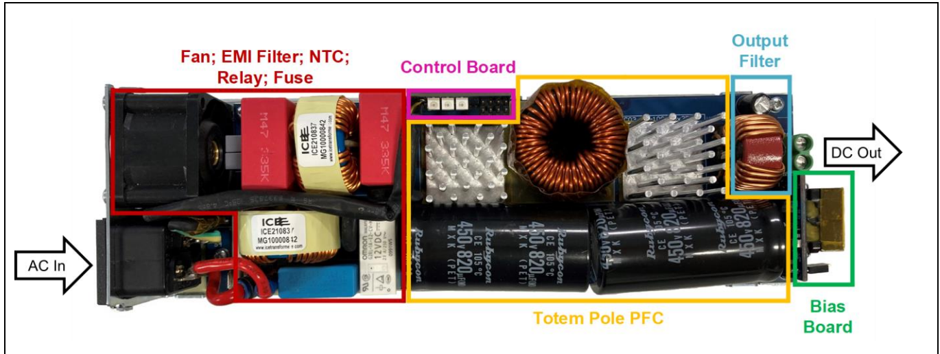
Figure 4 Placement of the different sections in the 3300 W bridgeless totem-pole PFC with Infineon CoolSiC™ 650 V MOSFET and XMC™ control
